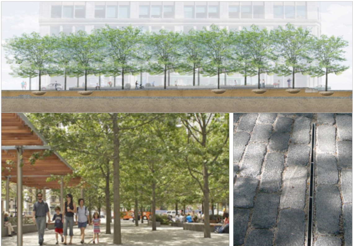
Top: Design section through plaza showing rootballs in SBSS
